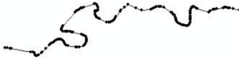
Figure 10 – Simplified line representation using BEND-SIMPLIFY algorithm and 20 m parameter among vertices – Number of resulting vertices: 147.
