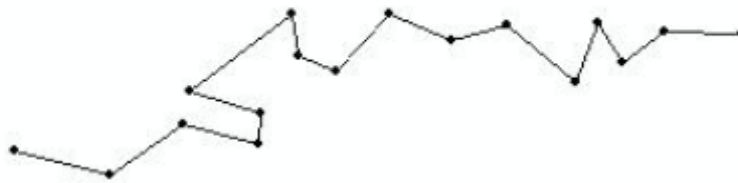
Figure 7 – Simplified line representation using POINT-REMOVE algorithm and 10 m parameter among vertices – Number of resulting vertices: 16.
